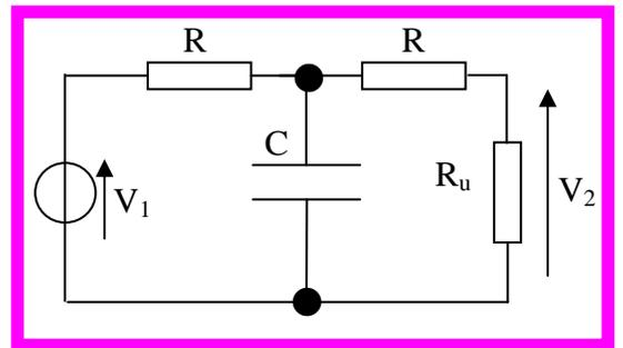
$$V_2 = E_{Th} \frac{R_u}{R_u + R_{Th}} \quad \text{soit} \quad V_2 = \frac{Z_c R_u}{R_u (Z_c + R) + R (Z_c + R) + Z_c R} V_1 \quad V_2 = \frac{R_u}{R_u (1 + \frac{R}{Z_c}) + R (1 + \frac{R}{Z_c}) + R} V_1$$
