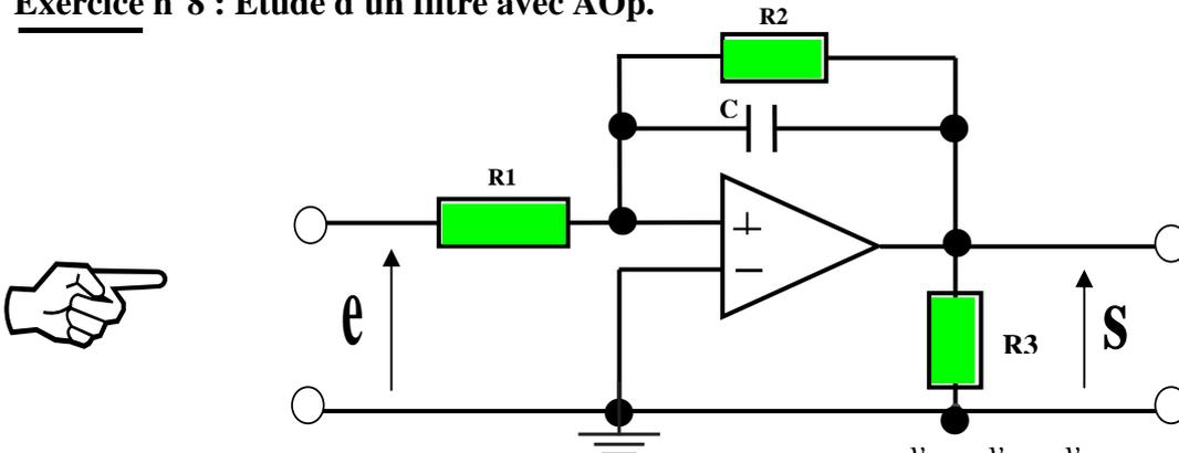
1°) Par application du théorème de Millman on trouve  $v_+ = \frac{\frac{v_s}{R_2} + \frac{v_s}{Z_c} + \frac{v_e}{R_1}}{\frac{1}{R_2} + \frac{1}{Z_c} + \frac{1}{R_1}} = 0 \implies \frac{v_s}{R_2} + \frac{v_s}{Z_c} + \frac{v_e}{R_1} = 0$
